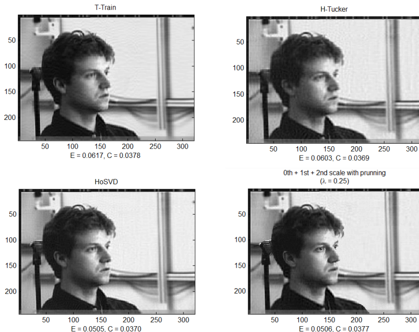
Fig. 9: Reconstructed frame samples from PIE data compressed by T-Train (top-left), H-Tucker (top-right), HoSVD (bottom-left) and pruned MS-HoSVD with 2-scales (bottom-right). 2-scale MS-HoSVD tensor approximation is obtained using \tau = 0.7 for each scale and \lambda = 0.25 .
