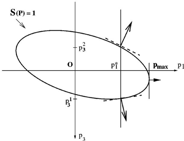
FIG. 1. The  $p_3$  components of outward normals at the two intersections on the convex slowness surface have opposite signs.
