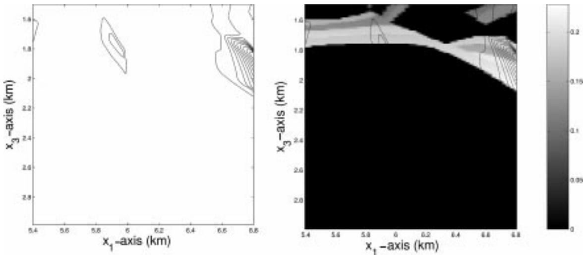
FIG. 6. Anisotropic effects on the wave propagation. (a) Nonzero contours of traveltime differences between the two Marmousi models concentrate on the region where  $\eta$  is larger. (b) Contours of traveltime differences overlaying  $\eta$  model; the maximum traveltime difference is 5.9 ms. See text for explanation of these differences.
