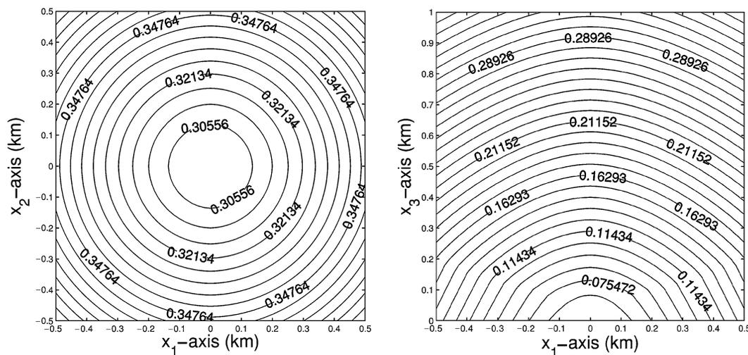
FIG. 3. 3-D homogeneous VTI model. The source is located at  $x_1 = x_2 = x_3 = 0.0$ . (a) Horizontal traveltimes slice at  $x_3 = 1.0 \text{ km}$ . Isochrons are circles because of the transverse isotropy. (b) Vertical traveltimes slice at  $x_2 = 0.30 \text{ km}$ .
