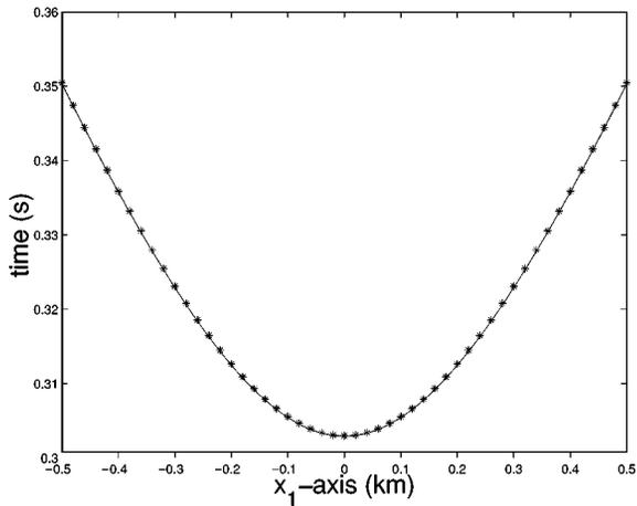
FIG. 4. Traveltime comparison at gridline  $x_2 = 0.2$  km,  $x_3 = 1.0$  km for 3-D homogeneous VTI model: ENO traveltime (\*) and analytic traveltime (-). ENO traveltime has almost the same accuracy as the analytic traveltime.
